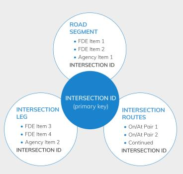
Using that single-point location and a primary key, the other key attributes needed to support the intersection MIRE data structures can be associated to the intersection.
